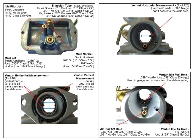
The "Slide Area" is the cylindrical space occupied by the carburetor slide as it moves up and down. Measurement surfaces of Tool A8 and A20 may not enter this space.
