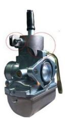
Optimization of the slide opening in Briggs & Stratton Kid Kart, Cadet, and Junior classes <u>is</u> permitted. The only allowable method of slide optimization is by removing material from the throttle cap area highlighted in RED. The use of multiple gaskets and/or machining of the slide is <u>prohibited</u>.
